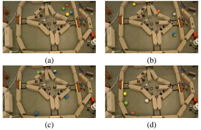
Fig. 15. A group splitting and coverage example: a) The 4 bodies begin together in the upper-right region; b) after 37 seconds the bodies begin to split; c) after 45 seconds bodies have split completely into independent regions; d) after 240 seconds bodies reconvene in the lower-left region.
