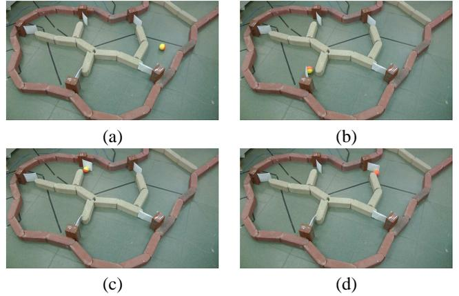
Fig. 11. “Patrol regions  $r_0$ ,  $r_3$  and  $r_1$ ”: a) The ball starts its route; b) after 107 seconds it has entered two new regions; c) after 212 seconds it has visited most regions; d) after 225 seconds, it completes a tour of all regions, and continues.
