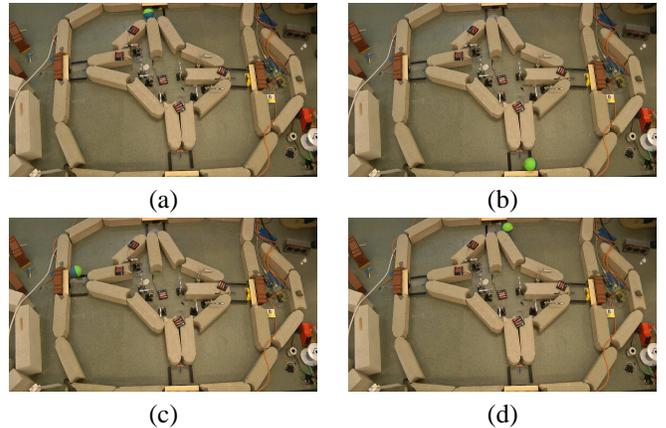
Fig. 12. A coverage task: a) The body crosses into the upper-left region; b) after 15 seconds, the body crosses into the lower-right region, completing the coverage; c) after 50 seconds, the body crosses into the upper-left region on the return trip; d) after 240 seconds, the body returns to the upper-right region.
