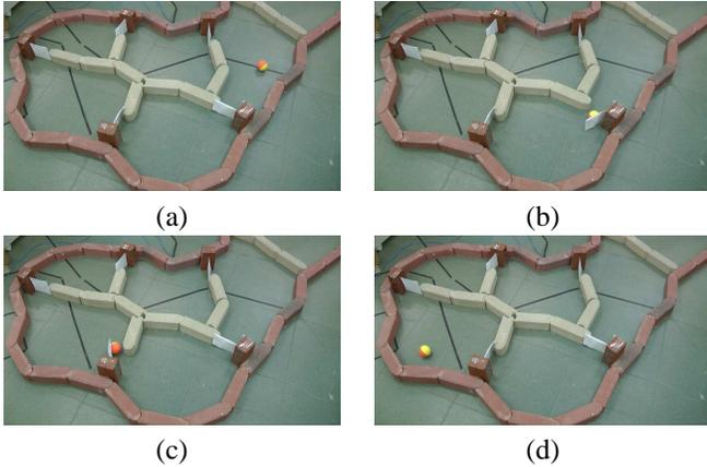
Fig. 10. “Starting in  $r_2$ , go to  $r_4$ ”: a) The weasel ball is placed initially in  $r_4$  (leftmost); b) after 30 seconds strikes gate  $d$  and enters  $r_3$ ; c) after 105 seconds it strikes gate  $e$  and d) moves into  $r_4$ , which completes the task.
